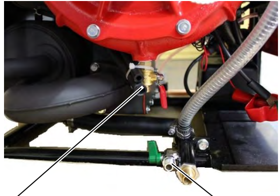
Pump drain cock
