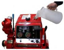
mark of the fuel gauge. Do not use mixed gasoline and Bio-gasoline.
