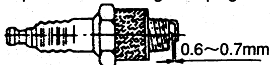
Gap of electrodes of ignition plug
